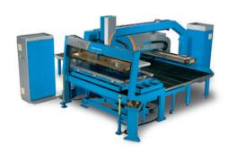
Component handling of the E5x can be automated with the **LST system**, which picks components from the machine and stacks them into programmed positions in the palletizing area. Further, the LST features an automatic skeleton removal function, and the entire working cycle of the machine becomes automatic. The LST can be equipped with several additional tables and integrated with the COMBO and Night Train automation systems.
